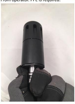
Insure Body and Chamber Are Fully Seated together.
